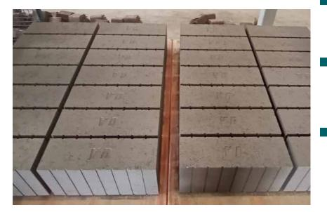
In traditional burnt clay bricks plaster is a must whereas in our bricks direct Paris can be applied.
